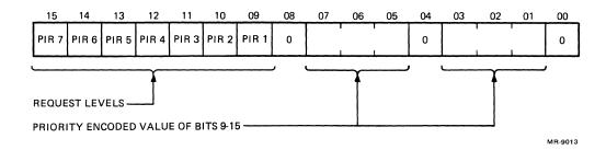
Figure 1-4 Program Interrupt Request Register (PIRQ)
