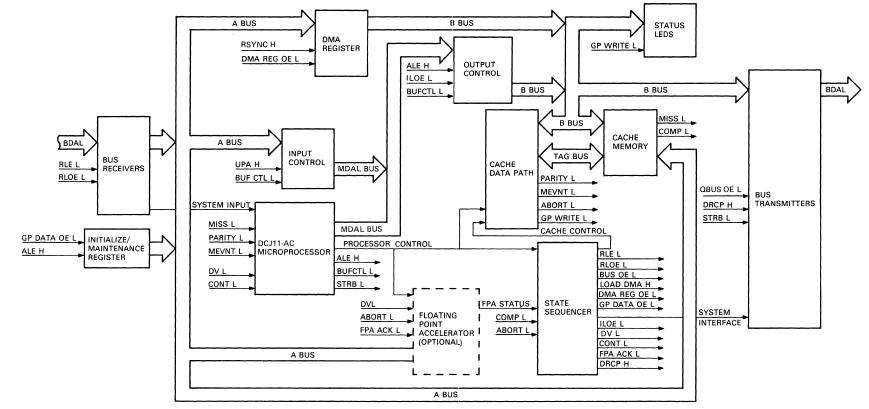
Figure 4-1 Functional Block Diagram
