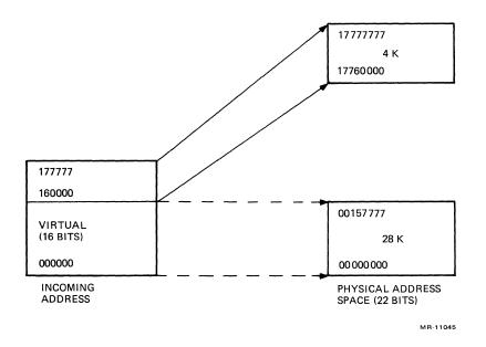
Figure 1-7 16-Bit Mapping
