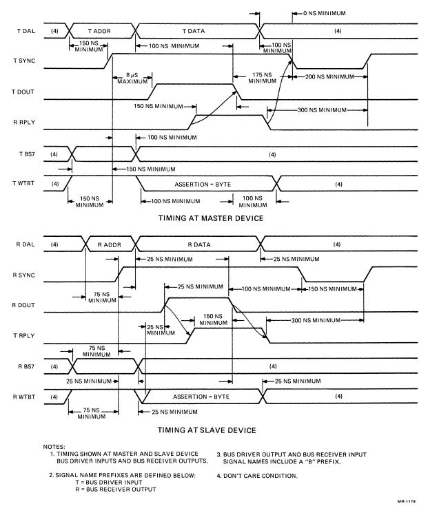
Figure 5-4 DATO or DATO(B) Bus Cycle Timing
