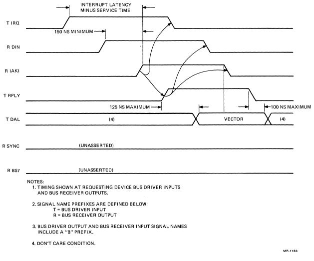
Figure 5-12 Interrupt Protocol Timing
