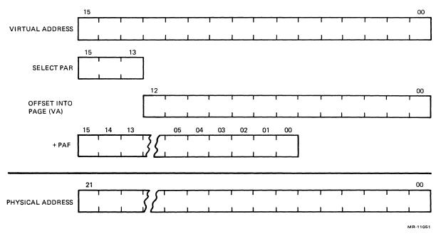
Figure 1-13 Construction of a Physical Address
