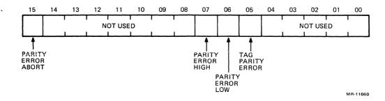
Figure 1-27 Memory System Error Register (MSER)
