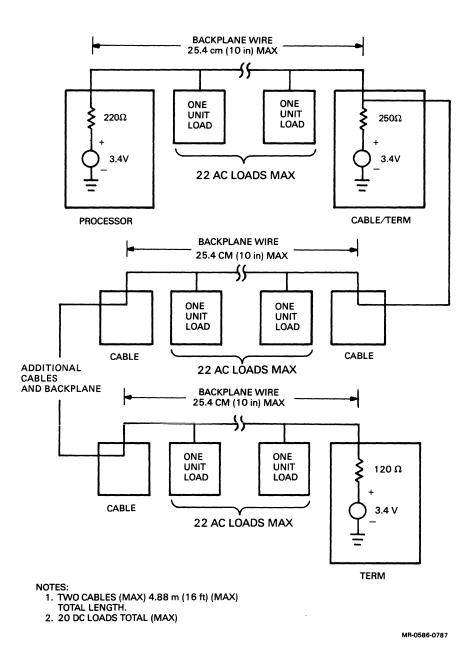
Figure 5-18 Multiple-Backplane Configuration
