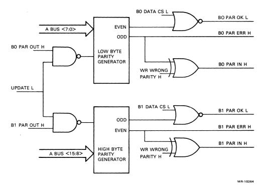
Figure 4-19 Cache Data Parity Logic
