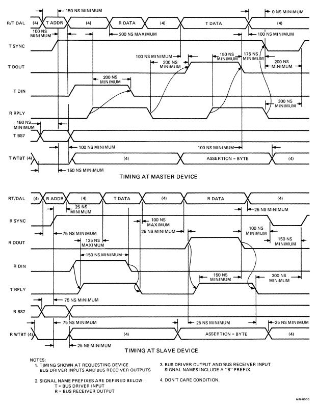
Figure 5-6 DATIO or DATIO(B) Bus Cycle Timing
