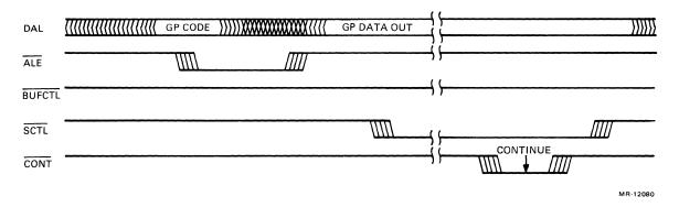
Figure 4-9 General-Purpose Write Transaction
