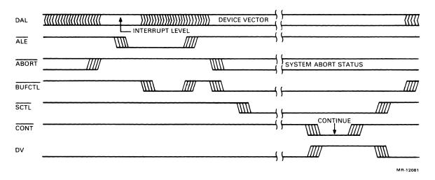
Figure 4-10 Interrupt Acknowledge Transaction
