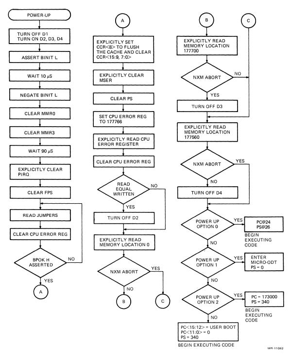
Figure 2-3 KDJ11-A Power-Up Sequence
