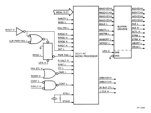
Figure 4-2 DCJ11-AC Microprocessor
