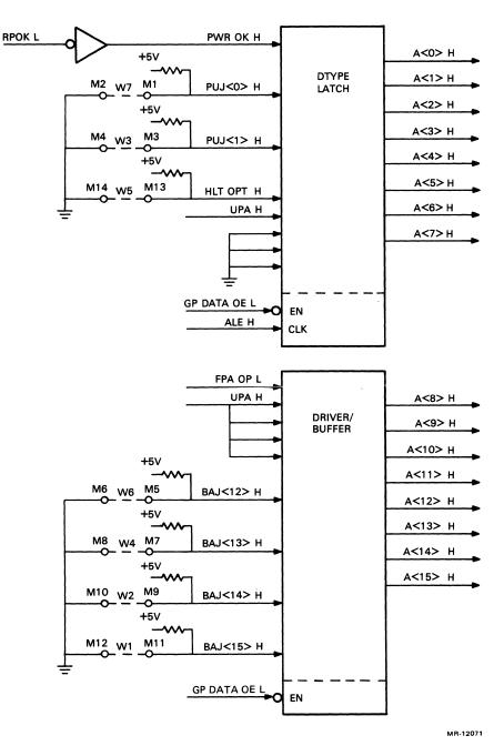
Figure 4-26 Initialization/Maintenance Register Logic
