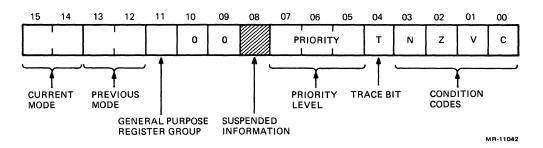
Figure 1-2 Processor Status Register
