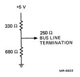
Figure 5-16 Bus Line Termination
