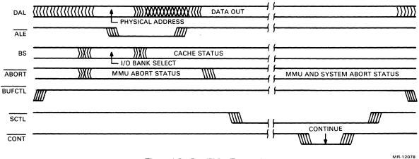
Figure 4-7 Bus Write Transaction
