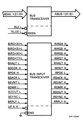
Figure 4-21 KDJ11-A Bus Receivers
