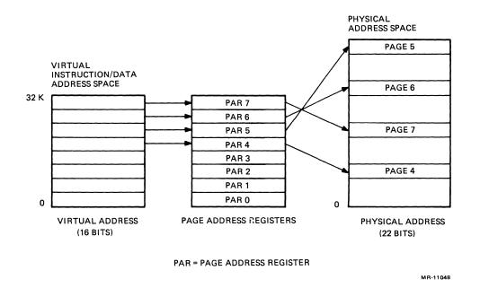
Figure 1-10 Virtual Address Mapping into Physical Address
