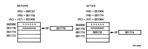
Figure 8-4 JSR Stack Condition Example
