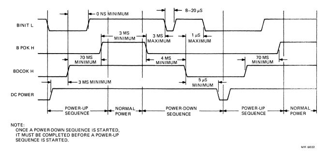
Figure 5-15 Power-Up/Power-Down Timing
