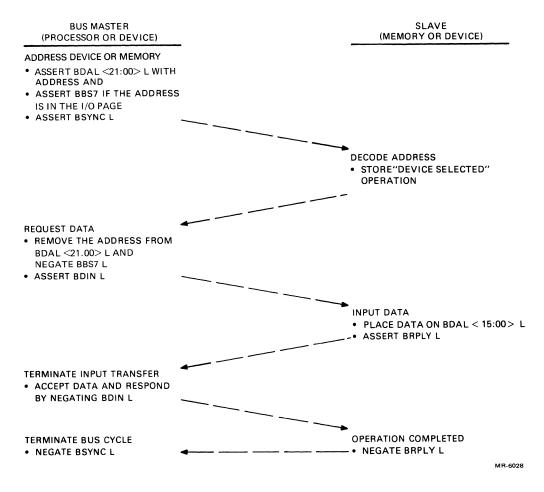
Figure 5-1 DATI Bus Cycle
