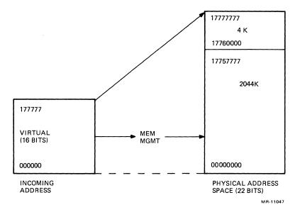
Figure 1-9 22-Bit Mapping
