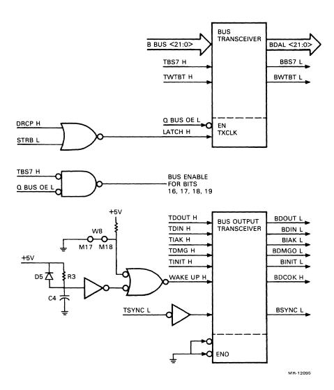
Figure 4-22 KDJ11-A Bus Transmitters
