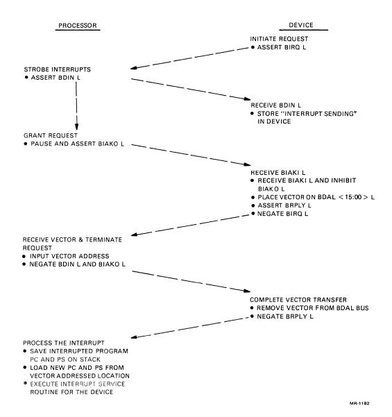
Figure 5-11 Interrupt Request/Acknowledge Sequence
