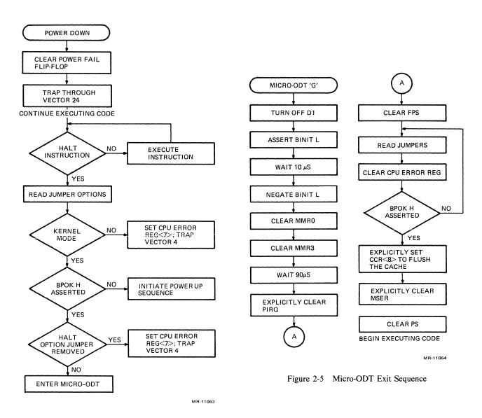
Figure 2-4 KDJ11-A Power-Down Sequence
