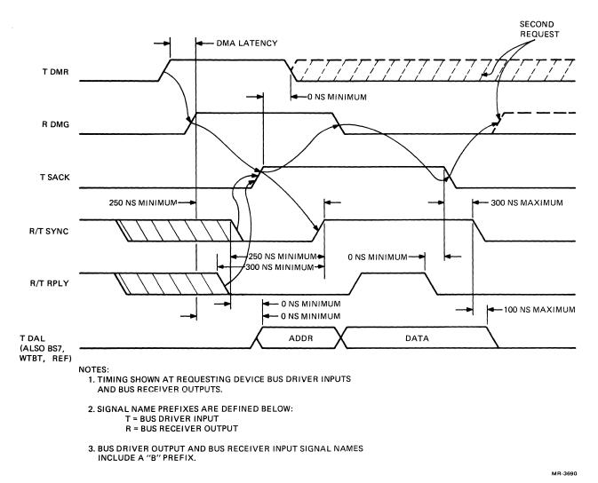
Figure 5-10 DMA Request/Grant Bus Cycle Timing
