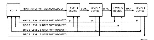
Figure 5-13 Position-Independent Configuration
