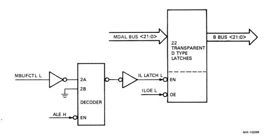
Figure 4-23 DCJ11-A Output Control
