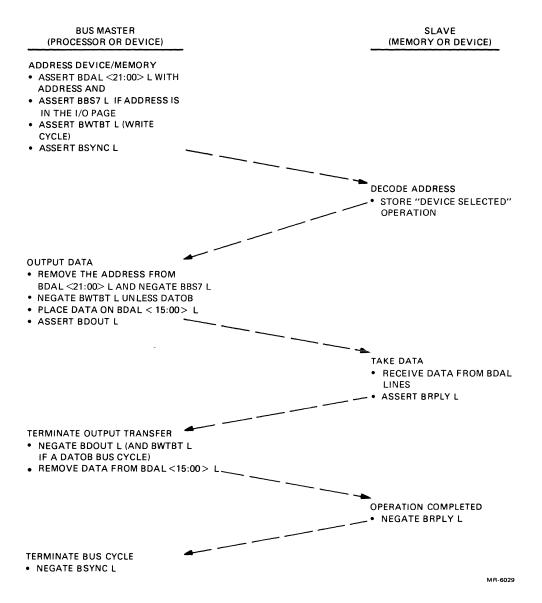
Figure 5-3 DATO or DATO(B) Bus Cycle
