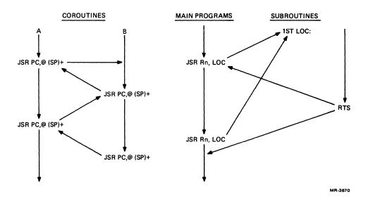
Figure 8-9 Coroutines Versus Subroutines
