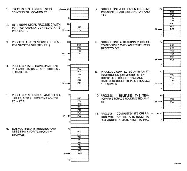
Figure 8-5 Nested Interrupt Service Routines and Subroutines
