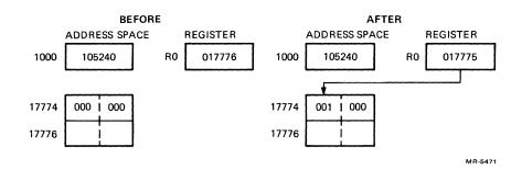
Figure 6-14 INCB -(R0) Increment Byte
