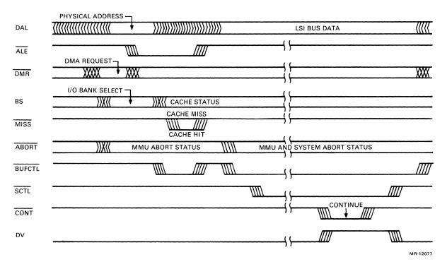
Figure 4-6 Stretched Bus Read Transaction
